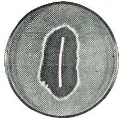
Photos show treated and untreated wire that has been subjected to fungus growths. (Left) Untreated, showing heavy fungus growth; inoculation with Chaetomium globosum No. 6205 spores. (Center) When properly treated with a fungicide, showing no growth, with wide zone of inhibition; spore suspension 1 of Chaetomium globosum . (Right) Properly treated with a fungicide, showing wide zone of inhibition; spore suspension of Trichoderma koningi .
