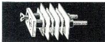
High voltage spring pile-up insulators of special heat treated Bakelite. Has minimum cold flow properties, low moisture absorption content and permits punching without cracks or checks.
