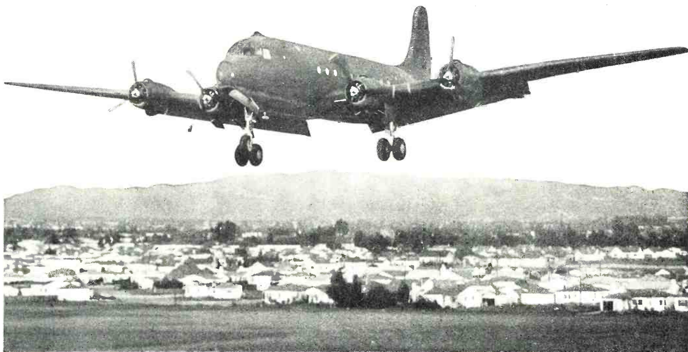
Douglas Skymaster. Army and Navy four-motored transport, with flaps lowered preparatory to landing.
