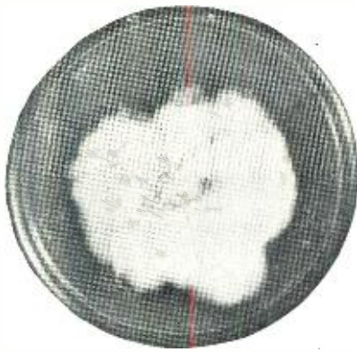
Photos show treated and untreated wire that has been subjected to fungus growths. (Left) Untreated, showing heavy fungus growth; inoculation with Chaetomium globosum No. 6205 spores. (Center) When properly treated with a fungicide, showing no growth, with wide zone of inhibition; spore suspension 1 of Chaetomium globosum . (Right) Properly treated with a fungicide, showing wide zone of inhibition; spore suspension of Trichoderma koningi .
